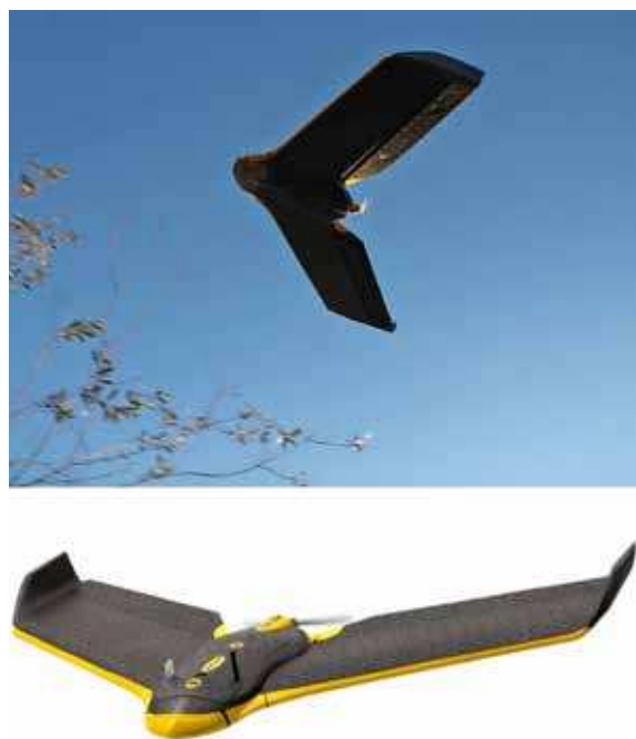
Figure 3.25: The flight equipment used at Crustumerium for landscape coverage is a SenseFly Ebee Parrot UAV with fixed wings. To carry out flights to monitor the archaeological excavations a hexacopter drone (Aibotix X6) was used.
