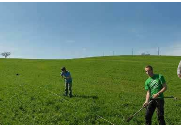
Figure 2.15: Coring by hand on the plateau of Crustumerium. The picture shows how coring data is acquired systematically, in straight rows at equal distance intervals.
