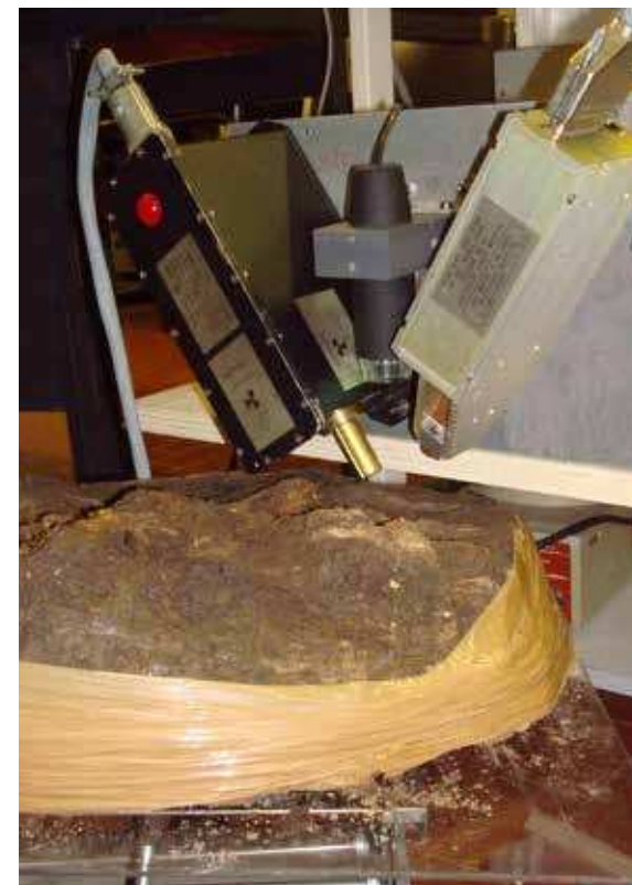
Figure 5.1: A soil block during XRF analysis.
