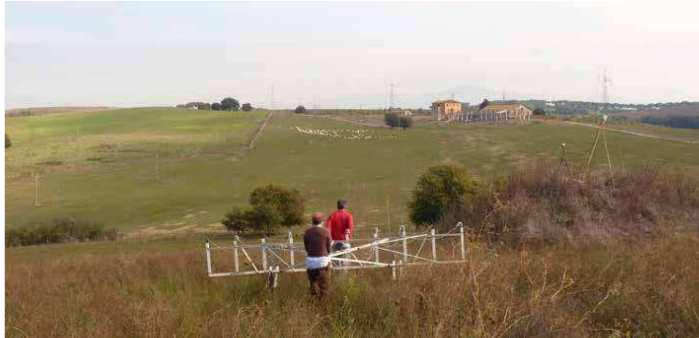
Figure 3.22: Technicians from Eastern Atlas performing magnetometric measurements with their custom built cart in the settlement area of Crustumerium.
